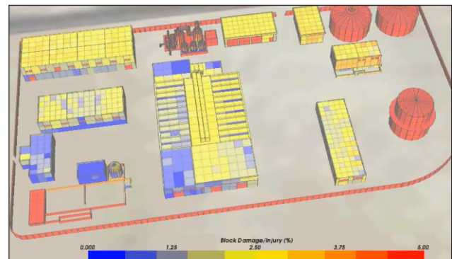
Building damage is displayed using color-coded 3D images.
